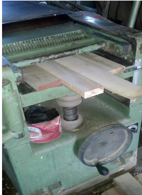
Plate 3.23 Planing of Planks with the Thickener Planer
