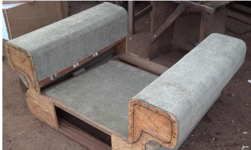
Plate 3.31 Covering with Fabric 3.18 Padding and Molding the Armrest and Backrest
