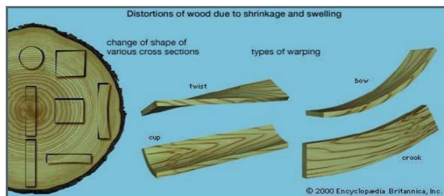
Figure 2.33: Distortion of wood due to shrinkage and swelling
