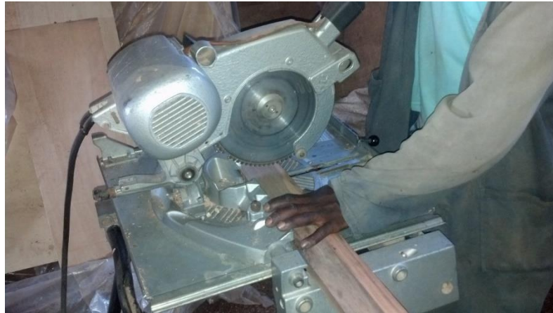
Plate 3.24 Cross-Cutting with the Cross-Cut Saw
