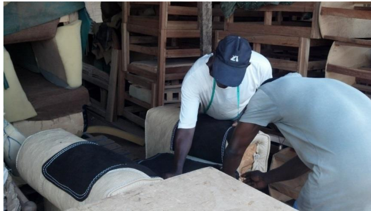
Plate 3.35 Fixing of Arm Rest and Seat 3.20 Carving of Face Plates and Back Rest Head Crown
